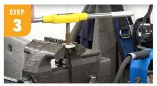
Using a hand drill and vise, drill 7/16" hole and thread with 1/4 NPT tap for the brass air filter. I used a 33/64" bit and 9/16" x 18" fine tap for the bottom fitting.
