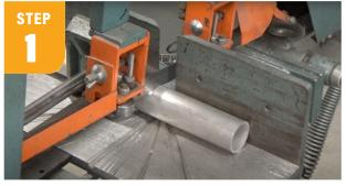
Take your round tubing and cut to desired length; remember to deburr the edges. Mine was cut to 5" long.
