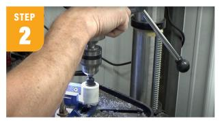
Using your 1-3/4" hole saw, cut two end caps out of the 1/4" aluminum. Sand or grind the rough edges if needed.
