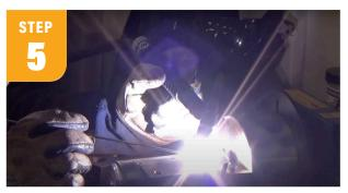
Take your mounting bracket and drill two 5/16" holes 1/2" from each end and 3/8" from the edge. Weld to the round tubing.
