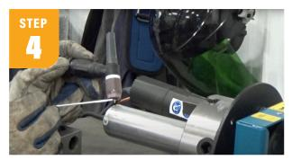
Set the Multimatic 220 AC/DC to 200 amps, 73% balance and frequency set to 90 hertz; then TIG weld the end cap to the round tubing.
